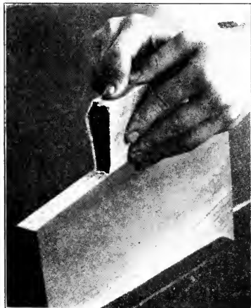
Fig. 125 - Sandpapering Edge with Narrow Block
